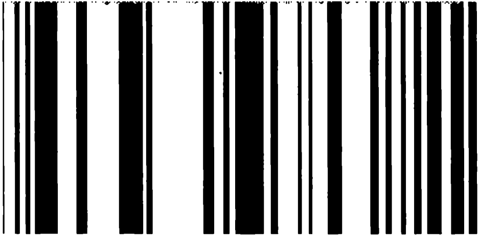
FIGURE 1.15 Temporal behavior of the k = 2, r = 2 code 56 totalistic rule of class II.
